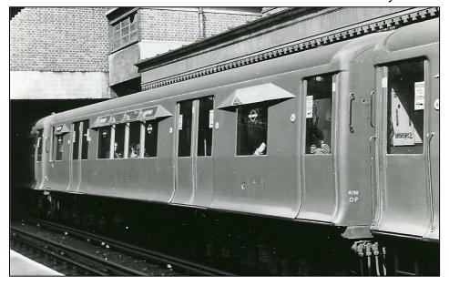
Left: OP Stock trailer 014081 on an inner rail Circle Line High working at Street Kensington in the early-1950s. As well as the passenger door open buttons (which were in yellow surrounds), labels were attached to the glass on passenger doors pointing to the button to be pushed. At that time, as well as bullseve no-smoking labels, white-onblue no-smoking labels were also to be found on some window toplights.
